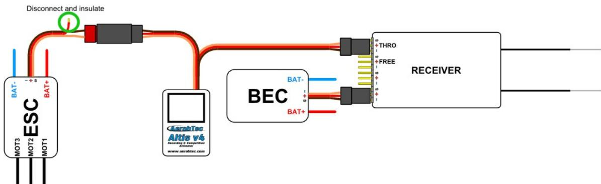
Fig 4: Connection of Altis v4 with BEC
