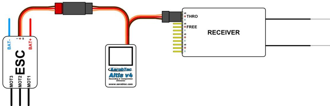
Fig 3: Connection scheme for competition use (ESC - electronic speed controller, THRO - throttle receiver channel)
