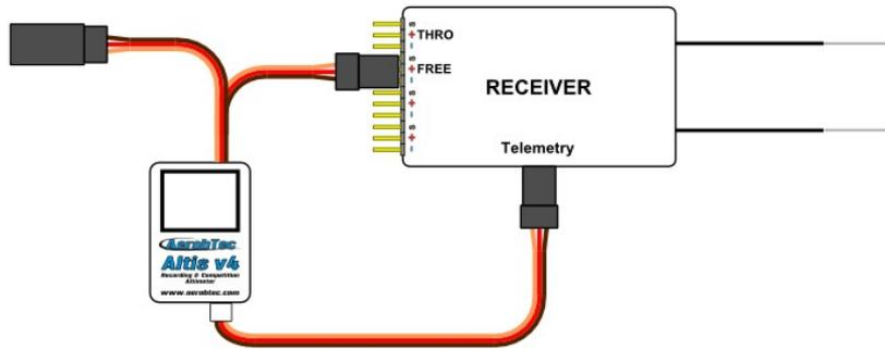
Fig 5: Telemetry connection
