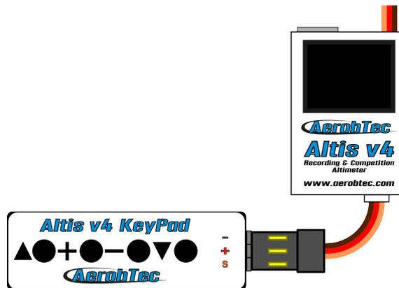
*Fig 15: Connection of Altis v4 Keypad*
